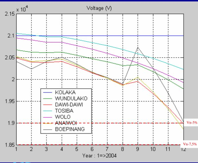
• Upgrade of all lines to 150  $mm^2$ • 900 kVAr of capacitors installed in Boepinang • 500 kW\_of additional installed capacity in Boepinang
